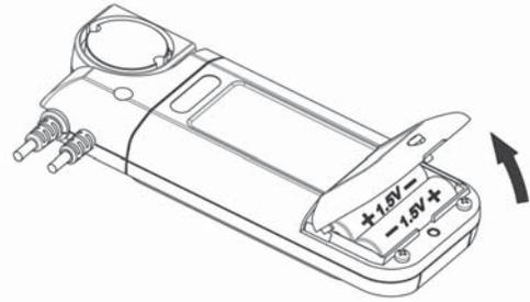
Replace with 2 new AA batteries (IEC LR6, NEDA 15A), observing correct polarity. Replace the battery cover.
